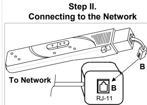
It is best to begin testing at the primary entry point of the local telephone line (Network Interface Test Jack). In this way you can determine if any problem is due to your provider or your own local installation. As shown, insert the free end of the adapter (B) into the modular RJ-11 telephone jack under test or Network Interface Test Jack (B).
