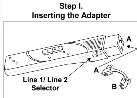
When you remove the cap from the unit, an adapter cord is pre-installed. It can be replaced or removed for the testing of extensions and cords. Begin by inserting, as shown, any end of the included adapter (A) into the modular RJ-11 Jack (A). Slide the Line 1/ Line 2 Selector Switch to the position of which line you are testing. If you are not sure, it's simple, just follow the next steps.
